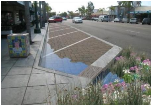
The Highway 101 Streetscape and Greenstreet projects improve water quality by reducing stormwater runoff through the use of pervious pavement and bioswales.
